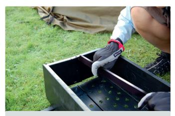
Put the support bar in the L-shaped hole.
